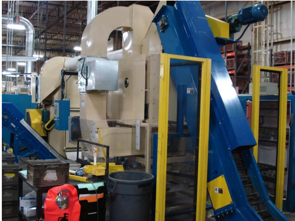
This is the infeed conveyor feeding the pre-heat tumbler. Part of the outer fencing has been removed for clarity.
